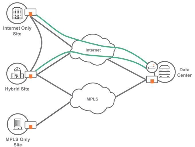
Figure 4. Hybrid SD-WAN network with SD-WAN overlay.
