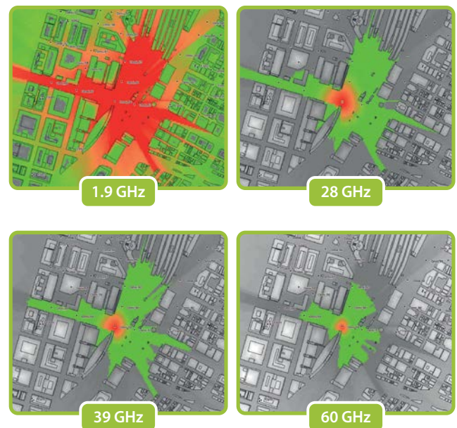
Figure 7. Evaluate the propagation characteristics of different frequency bands with Planet. These plots compare mmWave frequencies against a traditional 1900 MHz frequency using the Planet 3D Model.
